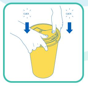
To permanently seal, push firmly at the two points indicated until clicks are heard and felt. A final visual check is recommended.
